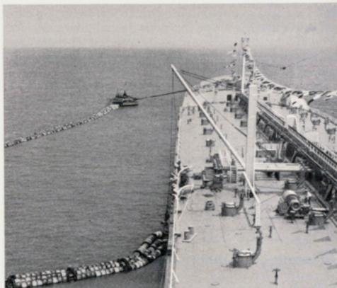
Fig. 220 Single buoy mooring
