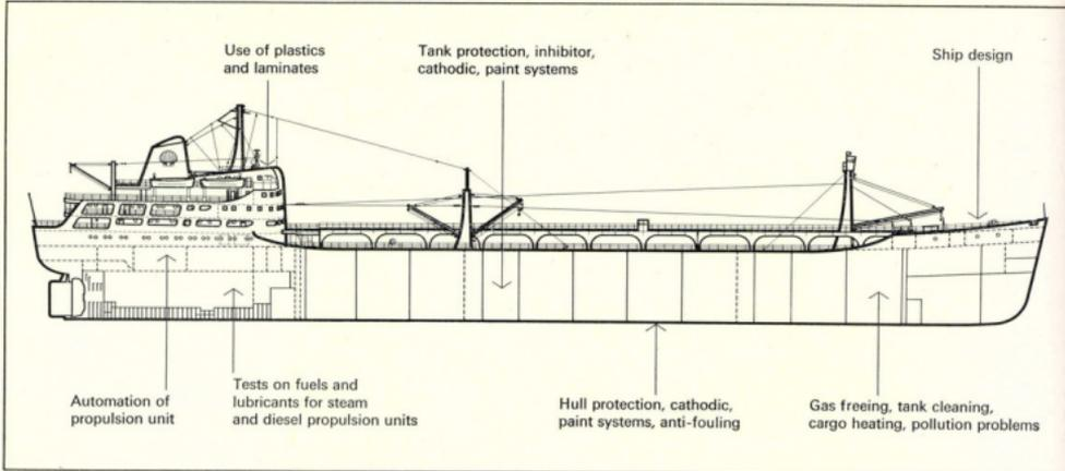
Fig. 250 Research problems connected with the tanker
