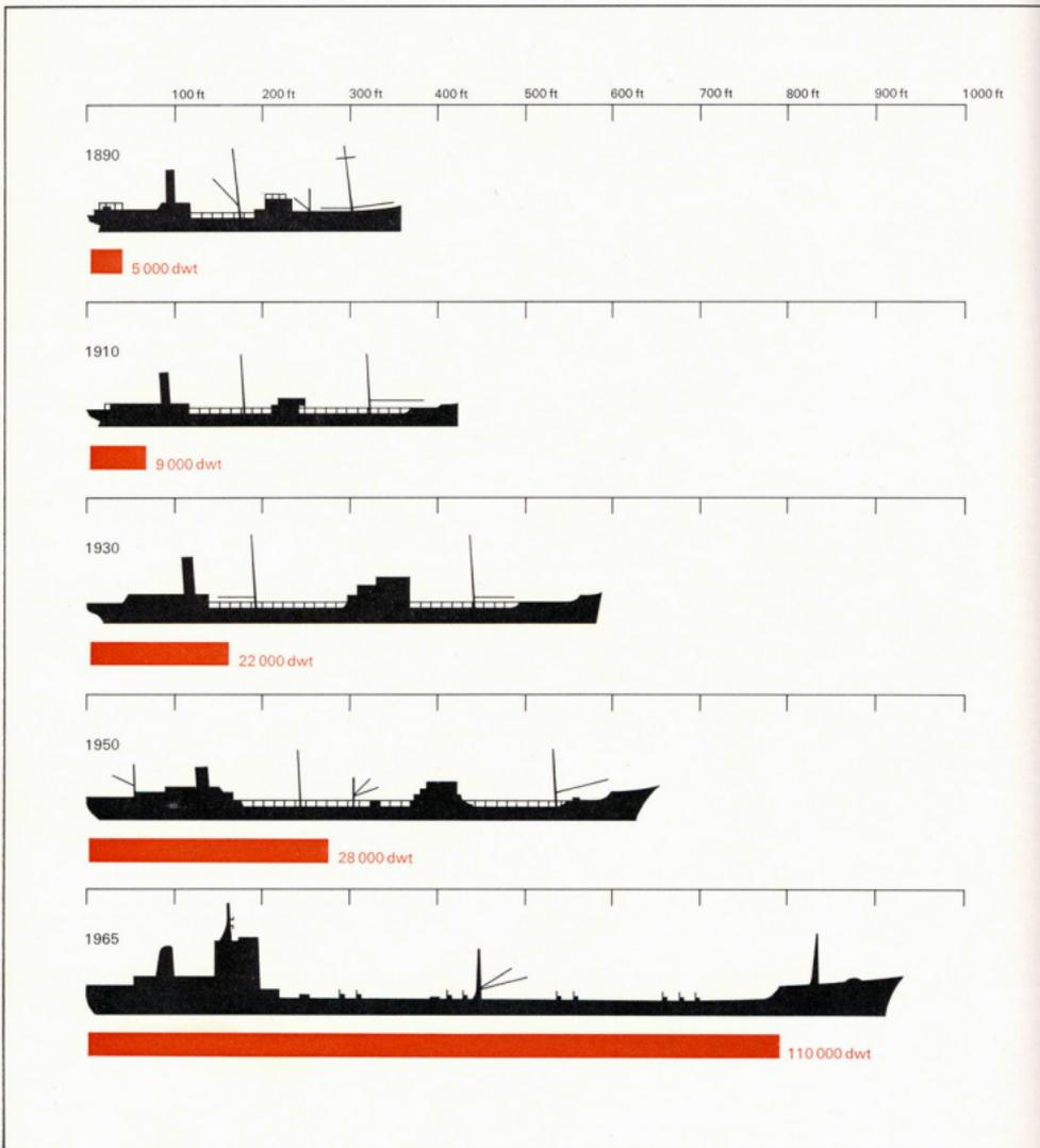
Fig. 213 Development in size, capacity and characteristic appearance of the ocean tanker
