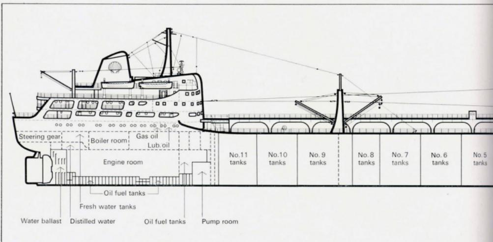
Fig. 218 Profile of a modern 22000 dwt general-purpose motor tanker
