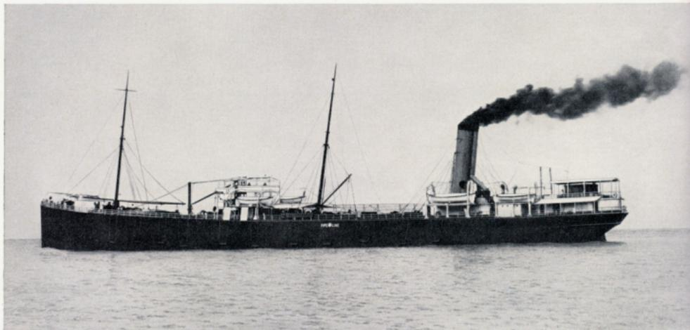
Fig. 211 Shell steam tanker *Volute*, 5670 dwt, built in 1893, a sister ship of ss *Murex*
