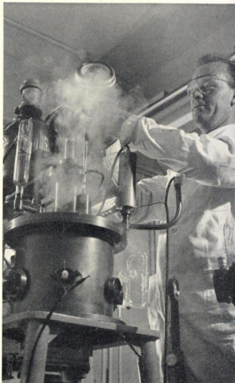
Fig. 251 The rotating cryostat used to isolate organic free radicals for further study
