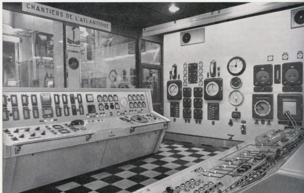
Fig. 219 Engine control centre on Société Maritime Shell's ss *Sivella*, 79327 dwt, built in 1963
